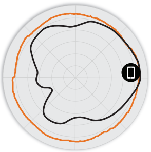
Figure 3 - T310d 5GHz Azimuth Antenna Patterns
